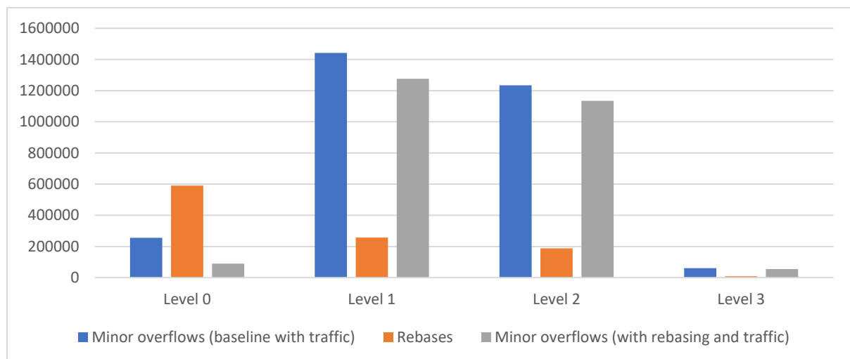
Figure 34 - Breakdown of minor overflows and counter rebases across the levels forming the integrity tree, for the loaded system; level 0 (i.e., leaf level) is used to protect system data; level 3 is the highest off-chip level, protected directly by the on-chip root
